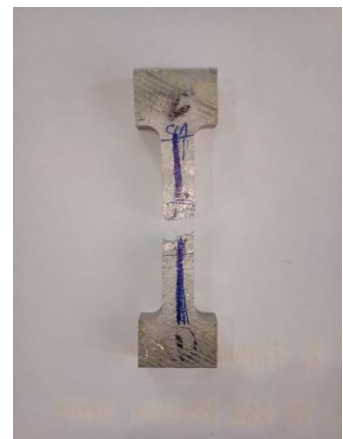
Figure 2: Tensile Test specimen
