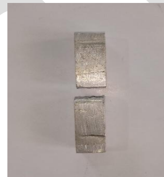
Figure 3: Impact Test specimen
